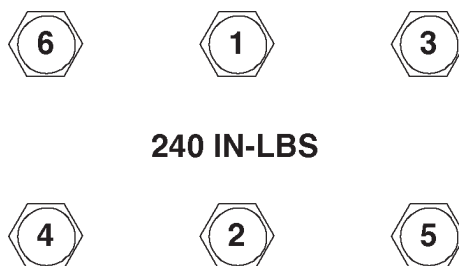
FIGURE 3. CYLINDER HEAD TORQUE SEQUENCE
