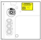
Each valve station incorporates [2] hydraulic ports and [2] coils. Manual override shafts are located in the center of the coils (see figure 4). Manual override decals are placed on each crane near the valve assembly. These decals provide a visual aid that helps the operator determine the function designations (Reference figure 3 & 5).
