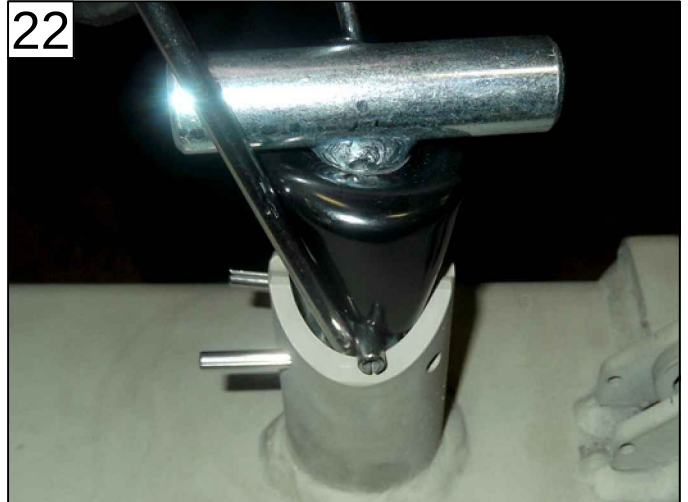
PUSH SPRING-LOADED WASHER DOWN
