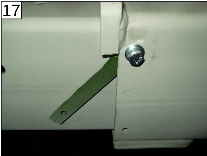
FASTEN NUT BAR RETAINERS ON BOTH SIDES PAGE 16 - ITEMS 6, 7, 8, & 9
