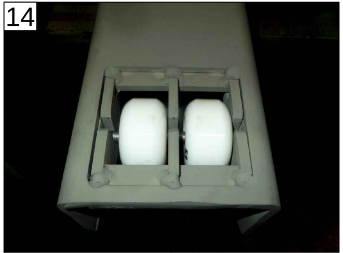
INSERT [1] SET INTO PULLOUT
