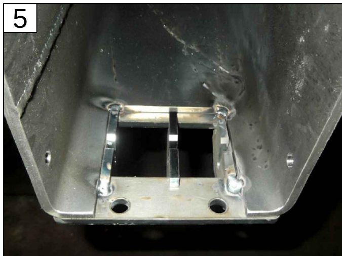
PLACE LAST AXLE SUPPORT CENTERED
