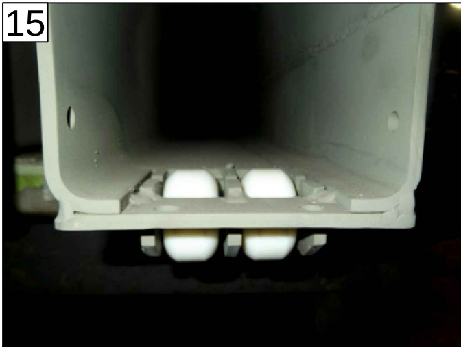
INSERT [1] SET INTO CROSSTUBE
