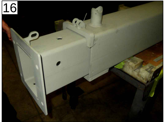
SLIDE PULLOUT INTO CROSSTUBE
