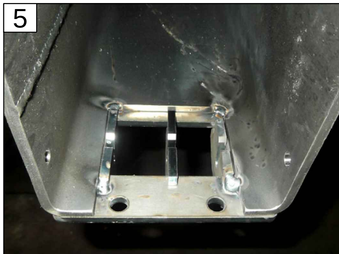
PLACE LAST AXLE SUPPORT CENTERED
