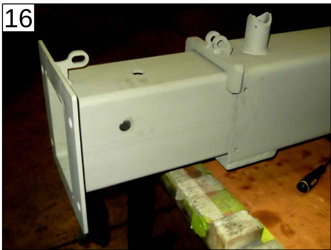
16 SLIDE PULLOUT INTO CROSSTUBE
