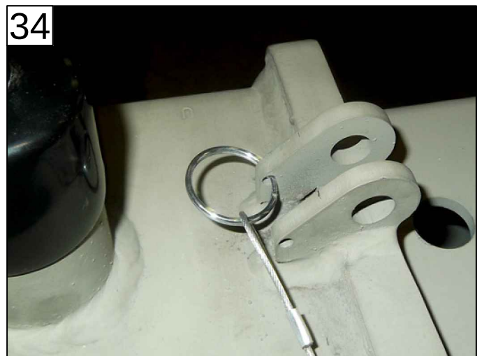
ATTACH SECURITY PIN'S KEY-RING ON EITHER TAB PAGE 21 - ITEM 12
