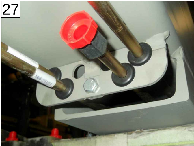
FASTEN CLAMP, ITEMS 26 & 27 REPEAT STEPS 25 TO 27 FOR OPPOSITE CLAMP
