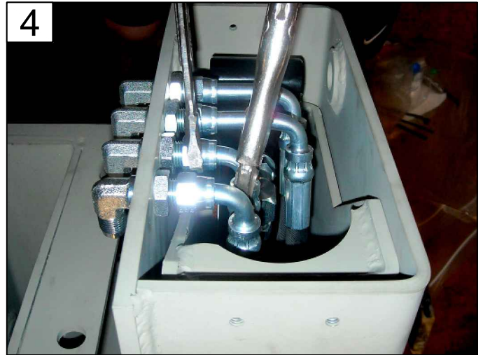
4 SEE HYDRAULIC MAPPING SECTION OF MANUAL REFER TO 'LETTER' TAGS ATTACHED TO PULLOUT HOSES
