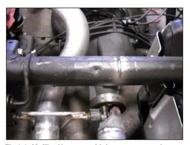
Fig 9.0 Muffler Hanger - with hanger removed
