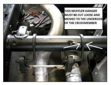
Fig 8.0 Muffler Hanger - Looking aft (Unmodified)
