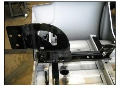
Fig 6.5 Upper Rear Hinge (Passenger Side) secured with original metric bed bolts; two places
