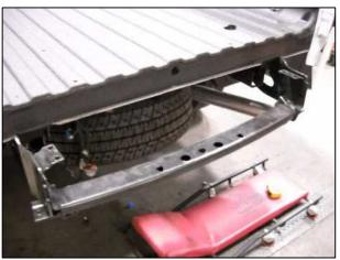
Fig 17.5 Rear Bumper Structural Member - dry fit to Upper Rear Hinges
