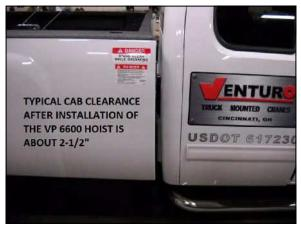
Fig 18.5 Typical Cab Clearance
