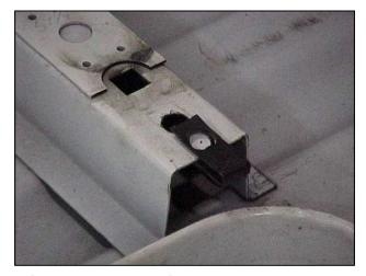
Fig 2 U-nut Installation
