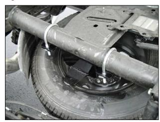
Fig 11.5 Install Tire Spacer / Scissor Rest
