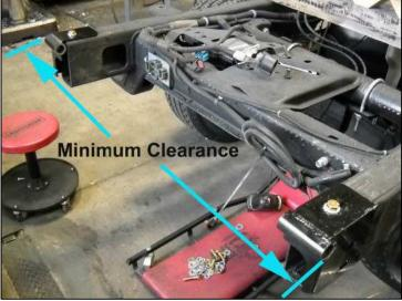
Fig 7.0 Lower Rear Hinge Assy positioned on end of chassis rail; illustrating the three bolts holes.
