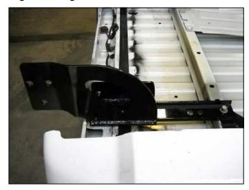
Fig 4.5 Upper Rear Hinge (Driver Side) secured using original metric bed bolts; two places.
