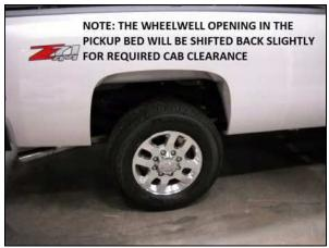
Fig 19.0 Wheelwell Displacement - Slightly Aft.
