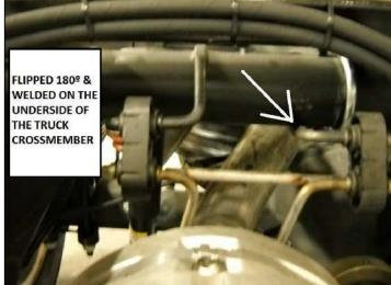
Fig 9.5 Muffler Hanger - with hanger flipped 180° and welded on the underside of the truck crossmember
