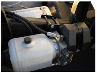
Fig 14.5 Hydraulic Power Unit Install Complete
