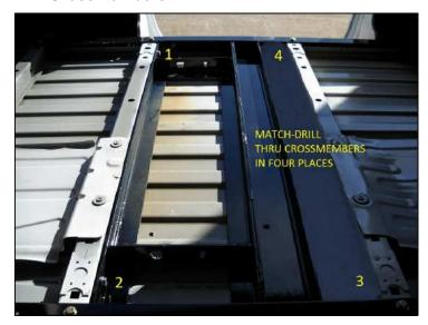
Fig 6.0 Upper Nest Installed between the 3rd & 4th bed crossmembers with 8ea Hex Head Cap Screws
