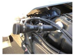
Fig 12.0 Typical Gas Filler Modification
