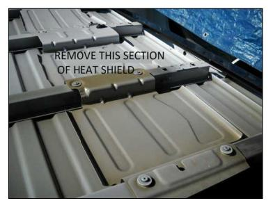
Fig 5.0 Remove Heat Shield between 3rd & 4th Crossmembers
