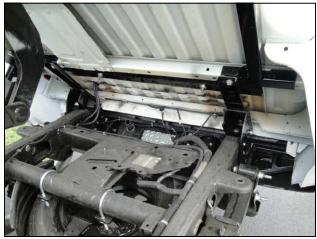
Fig 15.5 Pickup Bed Installation, Rear Hinges
